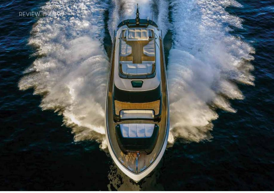
The AB 95 reaches up to 50 knots with three 2,000hp MAN V12 engines, two steerable waterjets and a central booster
