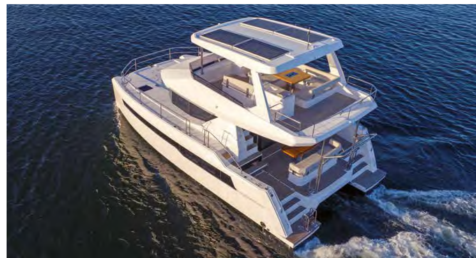
The Leopard 40PC can be fitted with twin 250hp, 320hp or 370hp engines, with the latter powering hull one to 23 knots in sea trials in South Africa
