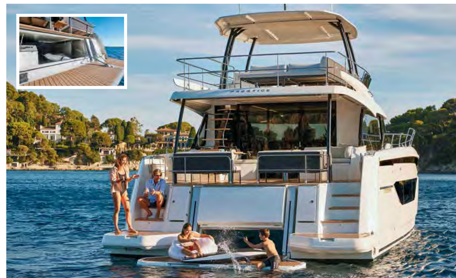
As well as a fun high-low platform for guests, the hydraulic platform can carry a tender and allow access to the toy garage (inset)
